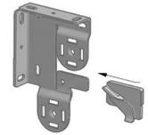
To remove the diverter a screwdriver can be used to wedge up from the bottom and release from the snap.
